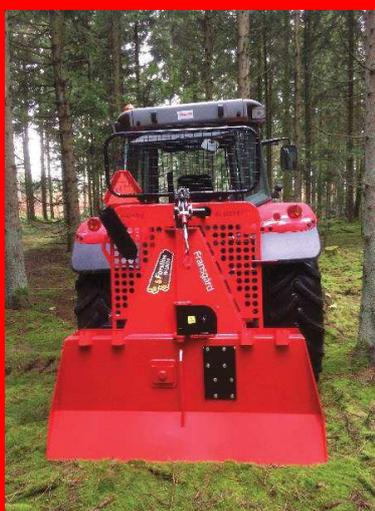
The unique design of the winch includes the smallest detail. The sturdy frame construction is made from special steel. A solid, wide blade/butt plate and lower pulley are standard. Chainsaw holder and trailer attachment are optional.
