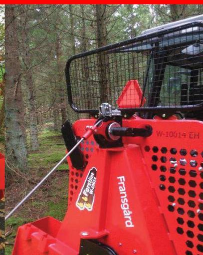
W-10014-EH with optional hydraulic device for unwinding wire rope, relieves the hard work, when pulling the wire out.
